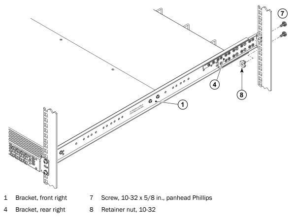
FIGURE 5 Attach the rear bracket to the cabinet rail
